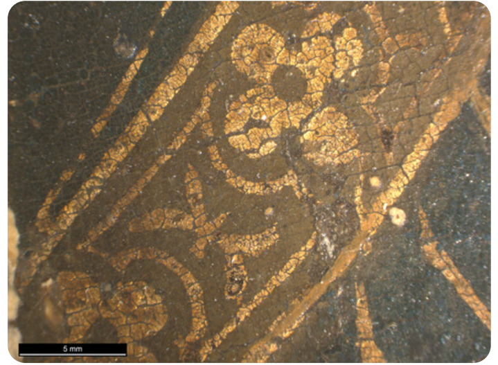
Technical Figure 20: Photomicrograph of mordant gilding in the Madonna's cloak. Badia a Isola Master, Madonna and Child , about 1300–1310, Indianapolis Museum of Art at Newfields, The Clowes Collection, 2009.52.
