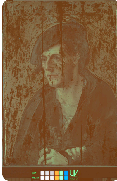
Technical Figure 23: Ultraviolet-induced visible fluorescence. Hans Schäufelein the Elder, Portrait of a Young Man , 1504, Indianapolis Museum of Art at Newfields, The Clowes Collection, 2004.159.
