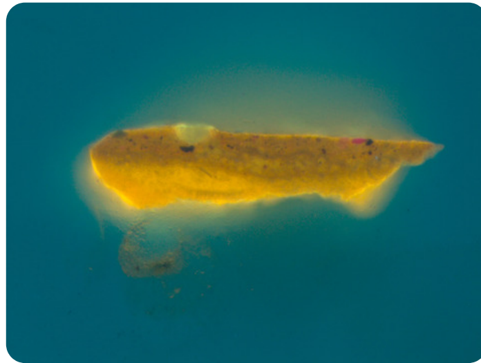
Technical Figure 17: Cross section sample 3c, photomicrograph showing fluorescent size layer at the bottom of the cross section, ultraviolet-induced visible fluorescence. Workshop of Rembrandt, Old Man with a Tall, Fur-Edged Cap , about 1650, Indianapolis Museum of Art at Newfields, The Clowes Collection, 2016.164..
