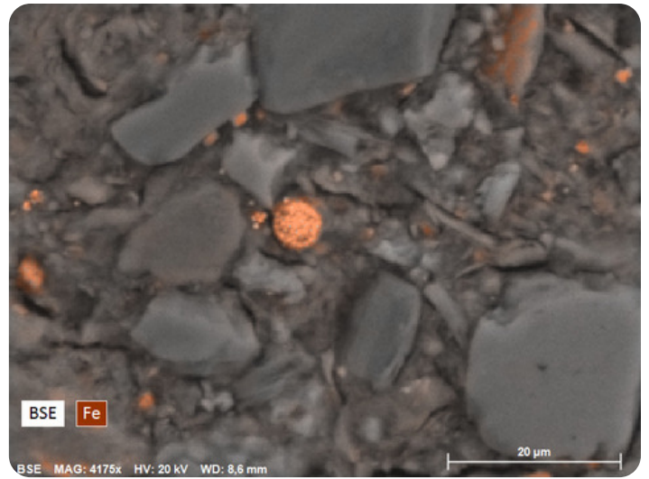
Technical Figure 17: BSE showing the presence of pyrite in the ground composition of cross section 3. The distribution of sulfur is shown in green and the distribution of iron is shown in orange. Jusepe de Ribera, A Philosopher, probably Euclid , 1637, Indianapolis Museum of Art at Newfields, The Clowes Collection, 2000.345.
