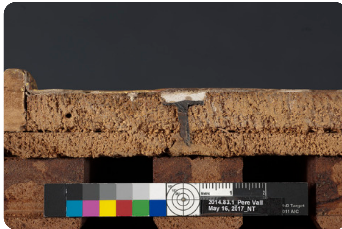
Technical Figure 11: Edge of the panel where the predella was sawn, revealing the cross section of an original nail used to attach the engaged frame to the panel. Pere Vall, St. Michael and St. Amador , about 1410, Indianapolis Museum of Art at Newfields, The Clowes Collection, 2014.83.1.
